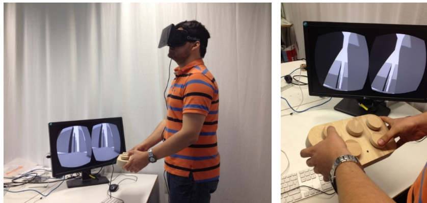
Fig. 2. Experimental Setup using Oculus Rift, Unity and a self-developed User Interface (based on Arduino Components)
